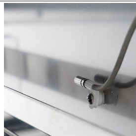
Internal cell probe for constant temperature monitoring
